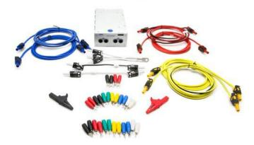
**The HVA Current Module** provides two 25 A sources at 150 VA each. When both sources are connected in parallel, 50 A at 300 VA continuous power is produced. Transient mode extends power and range up to 90 A at 300 VA for 30 seconds. DC output is 50 A.
