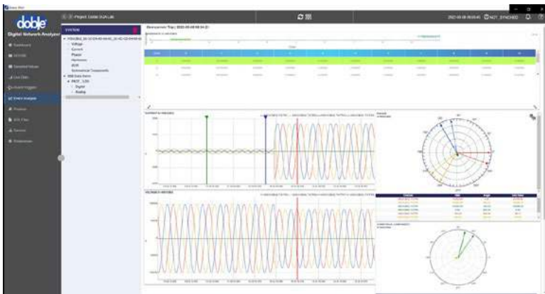
Configure the Live Data screen with oscillography, metering, and/or tabular UI elements to display live GOOSE and SV being polled from the network.
