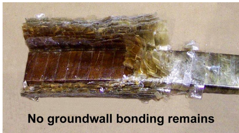
FIGURE 8: Dissection of the failed stator bar found no bonding between tape layers.
