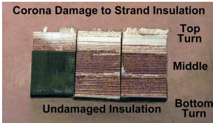
FIGURE 10: Additional cuts along the failed coil found internal corona had destroyed most strand insulation on the first turn near the machine bore.
