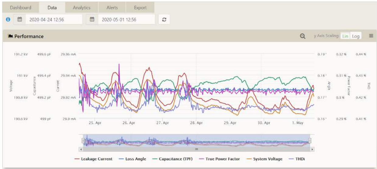
Figure 73 - Bushing Monitor Measurements
