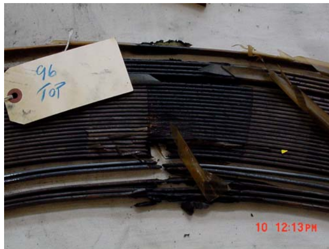
EVIDENCE OF DISCHARGE ACTIVITY ON A DISK FROM A FAILED TRANSFORMER FIGURE 2
