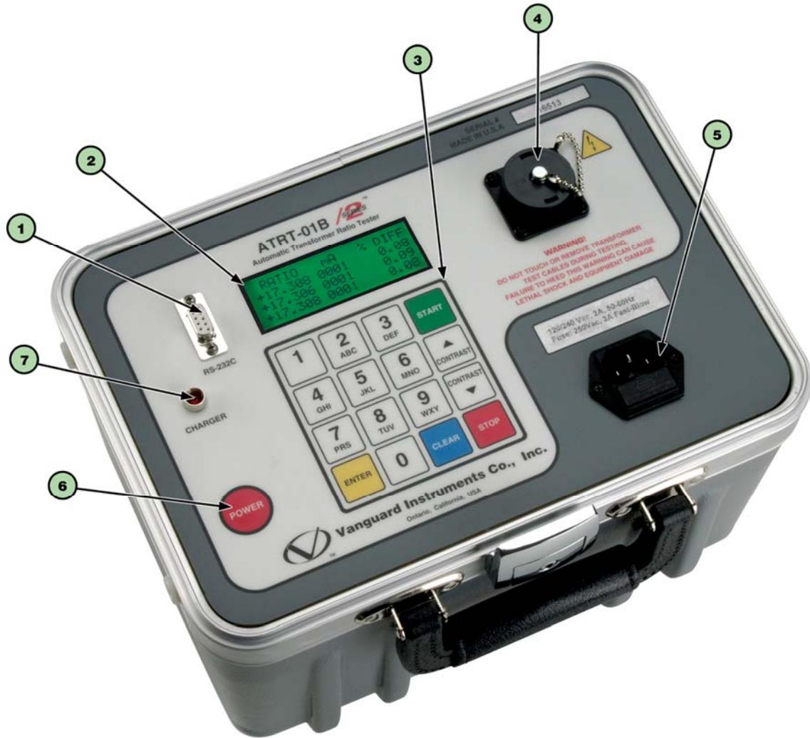
Figure 2. ATRT-01B S2 Controls and Indicators
