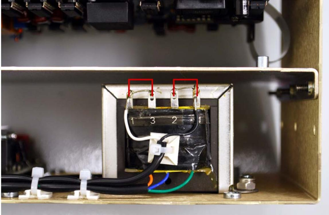
Figure 5. ATRT-01 S2 100 – 120 Vac Jumper Settings
