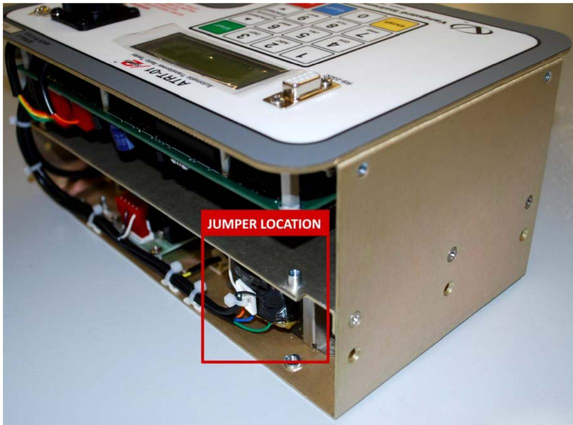
**Figure 4. ATRT-01 S2 Voltage Selection Jumper Location**
