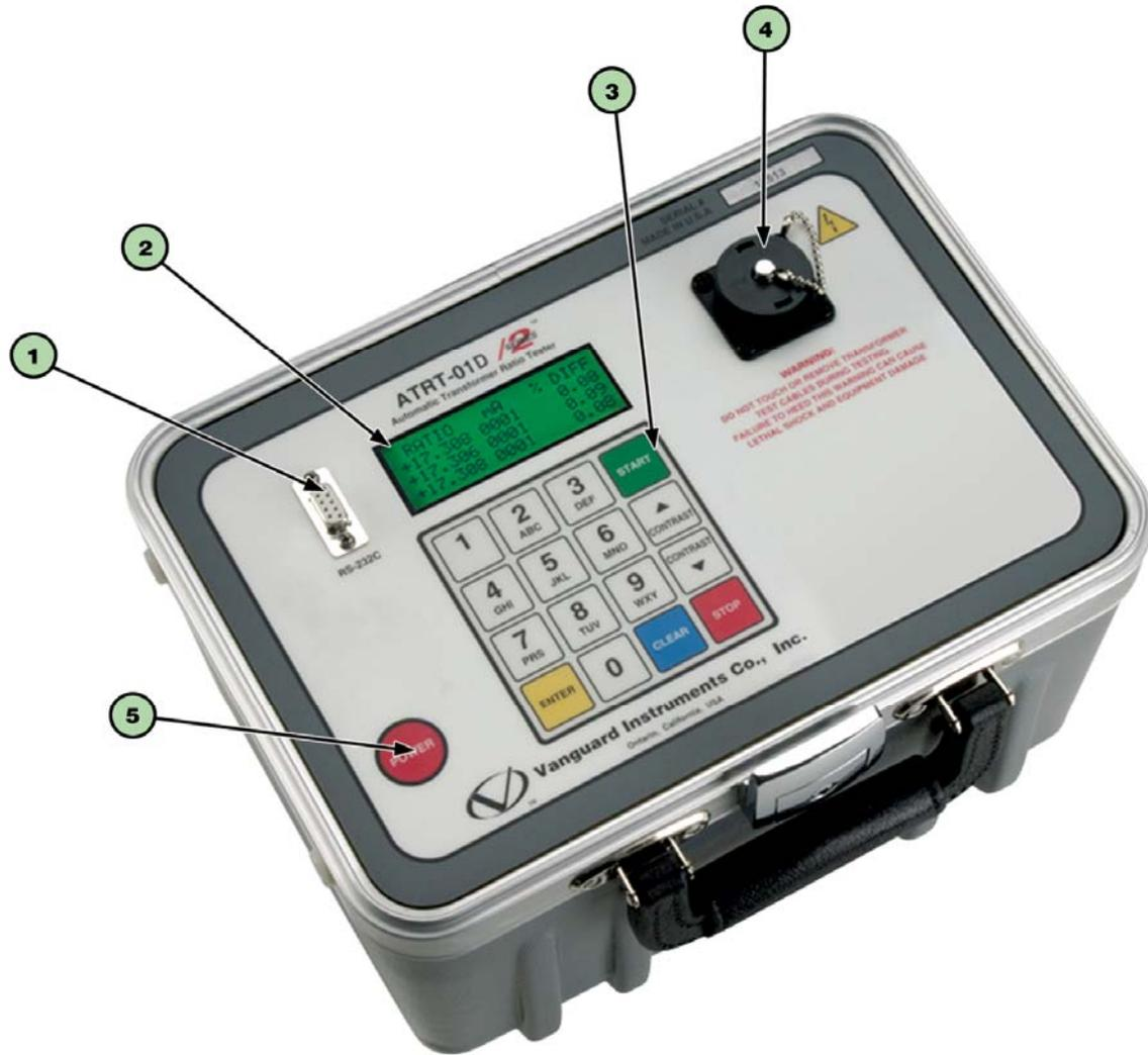
Figure 3. ATRT-01D S2 Controls and Indicators
