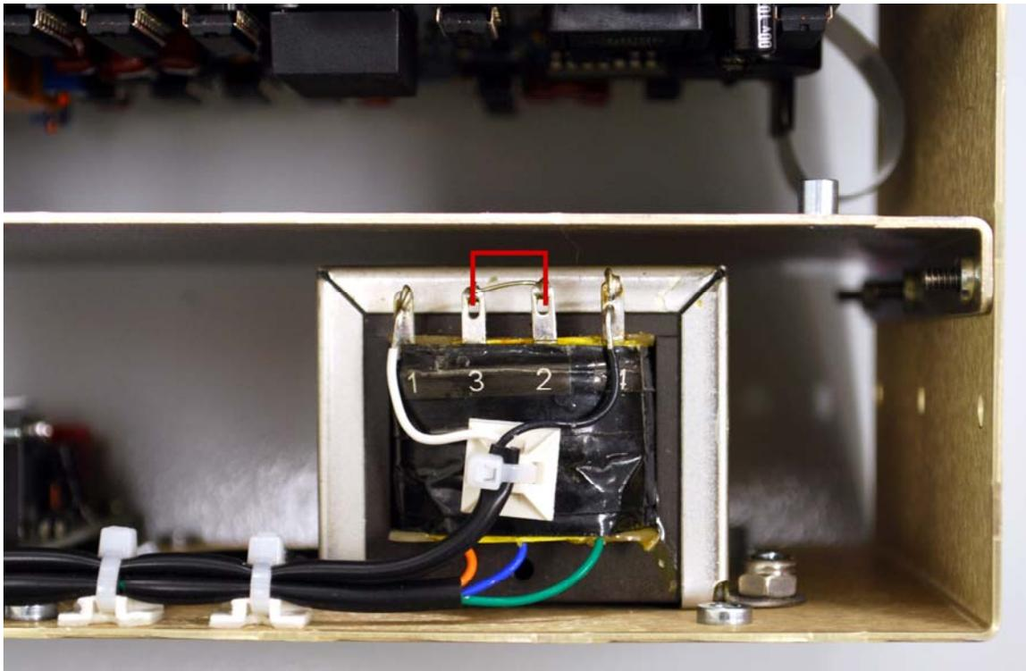
Figure 6. ATRT-01 S2 200 – 240 Vac Jumper Settings
