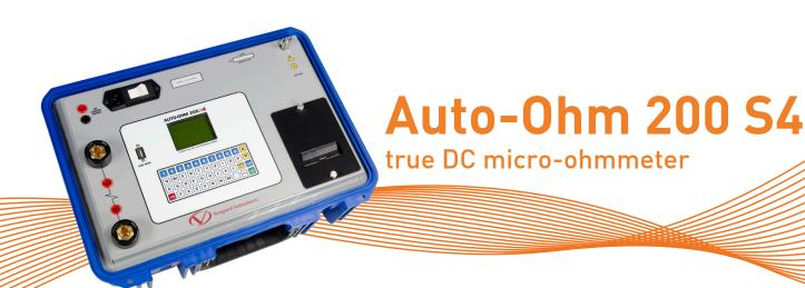
The Auto-Ohm 200 S4 is Vanguard's fifth generation, microprocessor-based, true DC micro-ohmmeter. It is designed for testing EHV circuit-breaker contact resistances, bushing contact joints, welding joints, or for any low-resistance measuring application. This high current and very lightweight (19.8 lbs/ 8.9 Kg) micro-ohmmeter is designed to meet the IEEE C37.09 requirement for testing circuit breaker contact resistance.
