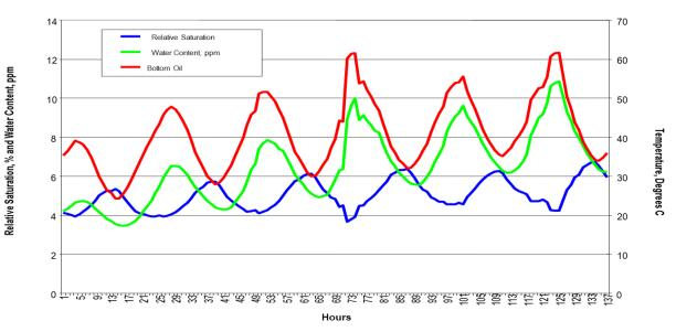
The dielectric strength of a insulating liquid correlates well to the relative saturation as opposed to the concentration level in ppm
