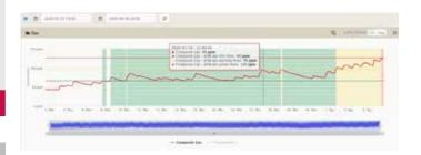
Intuitive user interface showing rising composite gas levels (solid red line) overlaid with alert limits (dotted green, yellow and red lines) and current alert state of the monitor (green, yellow and red backgrounds). The monitor has just reached ACTION (red level alert) so the background is now red.
