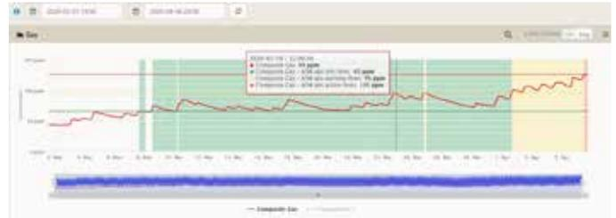
Intuitive user interface showing rising composite gas levels (solid red line) overlaid with alert limits (dotted green, yellow and red lines) and current alert state of the monitor (green, yellow and red backgrounds). The monitor has just reached ACTION (red level alert) so the background is now red.
