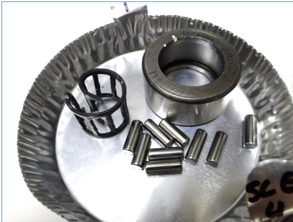
Rollers and Race from Circuit Breaker 1-1 Bearing Figure 9
