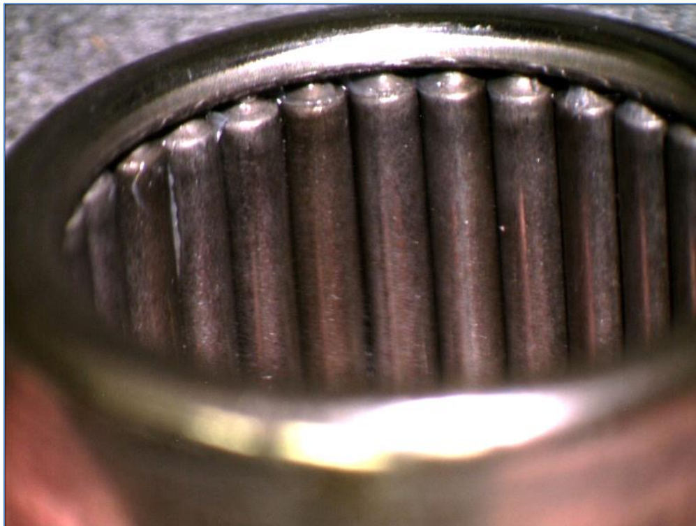
Needle Roller Bearing Circuit Breaker 1-4 Installed in 1997 Figure 10
