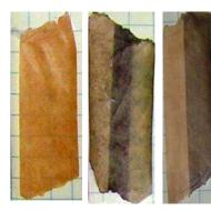
Paper with no or dull deposits From left to right: No deposit, heavy dull deposit, and moderate dull deposit PASS
