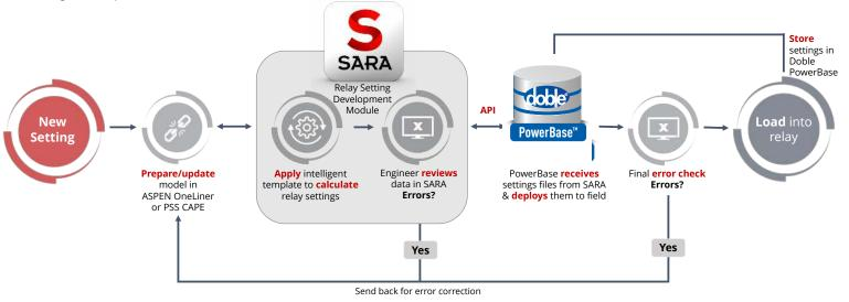
**Complying with R1** begins by preparing the model within a short circuit program such as ASPEN OneLiner or PSS CAPE. The latest data can be automatically retrieved from Doble PowerBase, minimizing time spent preparing new settings.
