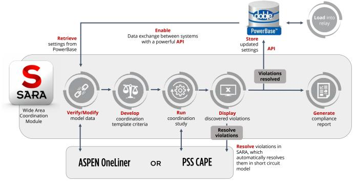
Complying with R2 begins by verifying the model. After SARA retrieves the latest settings from Doble PowerBase, it can then import this data into the short circuit program to verify the model, eliminating the need for manually transporting data between the two programs.
