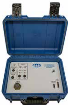
F5850 Test Interface for S&C IntelliRupter® PulseClosers®
