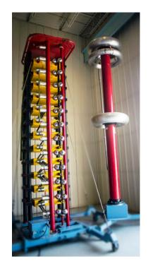
Design and manufacturing problems can cause premature equipment failure. To minimize that risk, Doble's high-voltage laboratory offers a wide range of qualification and acceptance tests for medium-voltage and high-voltage rotating machines.
