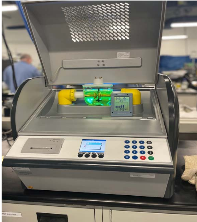
Figure 7: Dielectric Breakdown Voltage Test Set and Calibrated Digital Barometer
