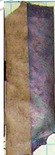
Figure 4c: Metallic Sulfide Deposit Paper from Doble CCD Test
