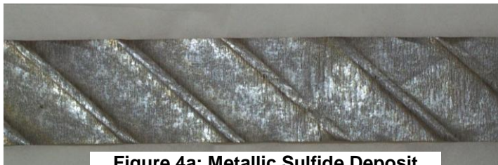
Figure 4a: Metallic Sulfide Deposit on Paper from Failed Winding
