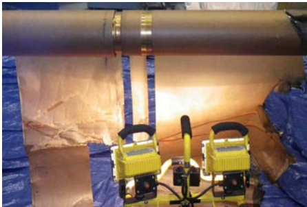
Figure 7. Partial core of a bushing showing tap foils
