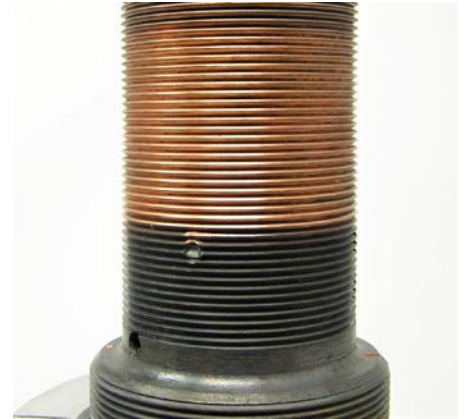
Figure 12. Copper sulfide formation on copper conductor
