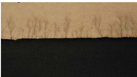
Figure 9. Partial discharge treeing from edge of ink layer
