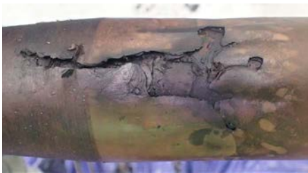
Figure 8. Arcing through core
