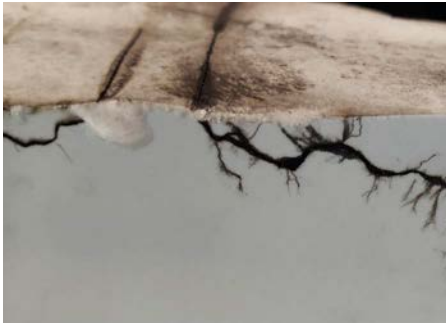
Figure 6. Arc tracking on internal porcelain
