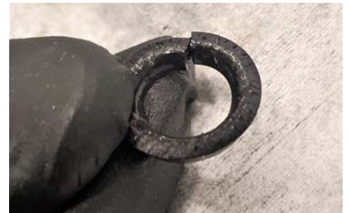
Figure 3. Broken and deteriorated oil fill plug O-ring
