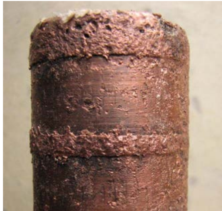
Figure 11. Pitting and melting of copper conductor
