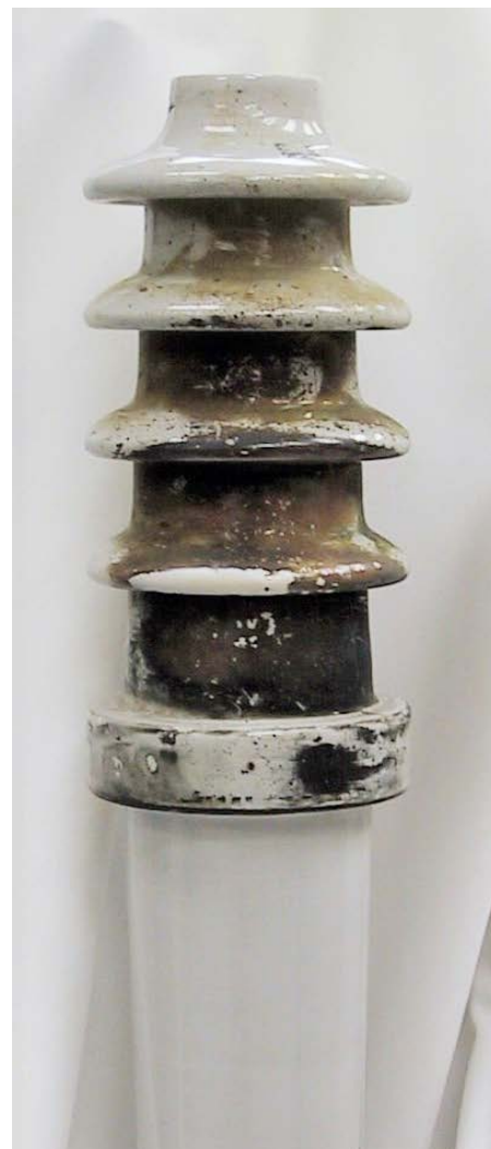
Figure 1. Hot oil and fire soot deposits
