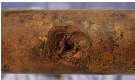
Figure 10. Arc hole through copper conductor
