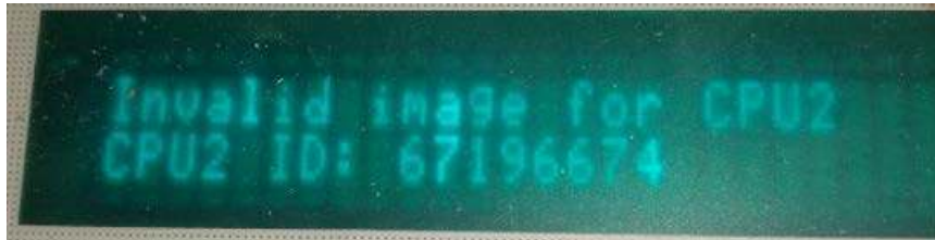
Figure 13. F6150 CPU2 instrument invalid-image error message after update
