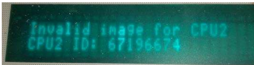
Figure 14. F6150 CPU2 instrument invalid-image error message after update
