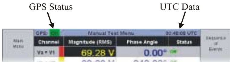
FIGURE 6.2 GPS STATUS DISPLAYS
