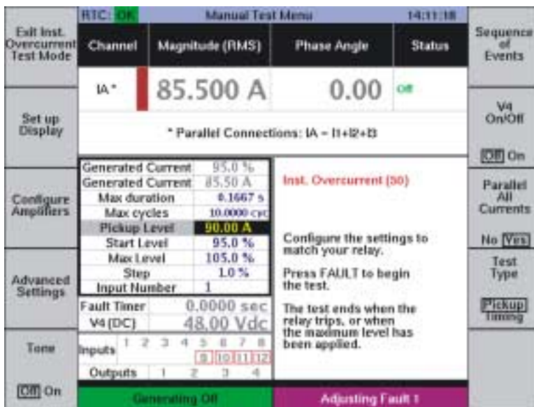
FIGURE 3.17 OVERCURRENT RELAY TEST MODE
