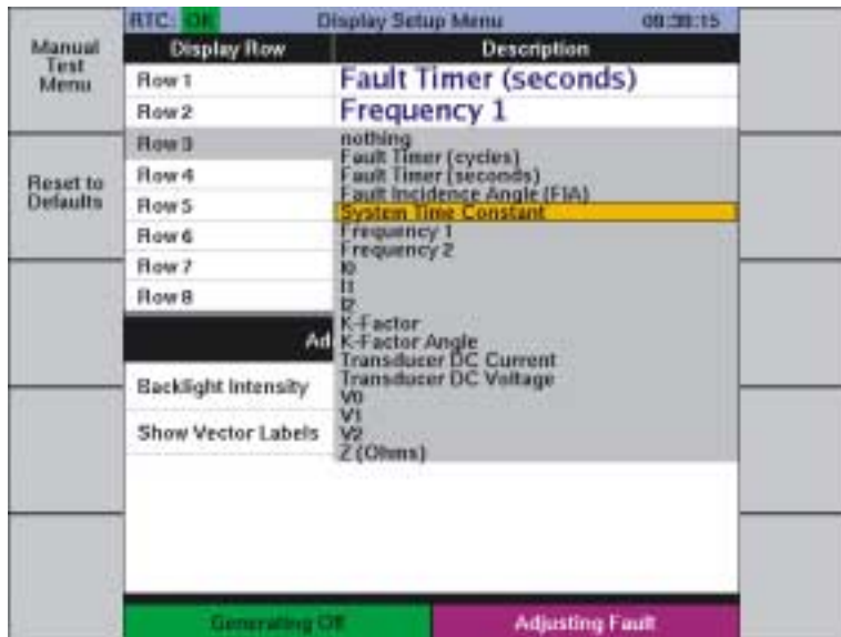
FIGURE 4.23 DISPLAY SETUP MENU
