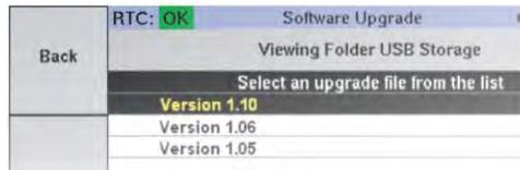
Press *Copy File From USB* [F10] and WAIT until the button turns from dark grey to light grey again. This loads the file into the MTS-5100's on-board files.
