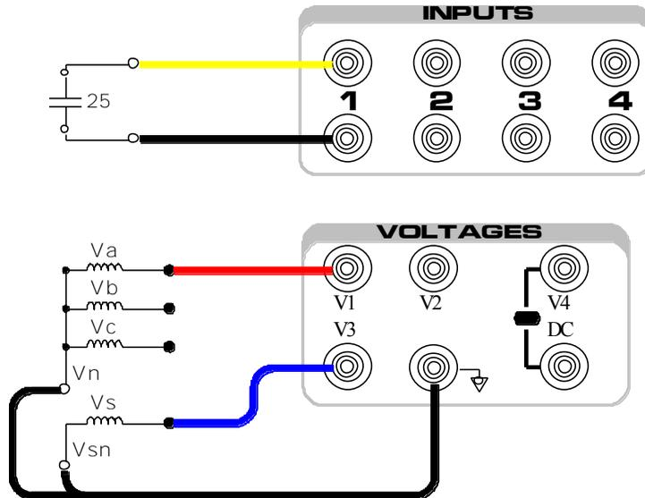
**Synchrocheck Relay: Wiring Type = Delta**
