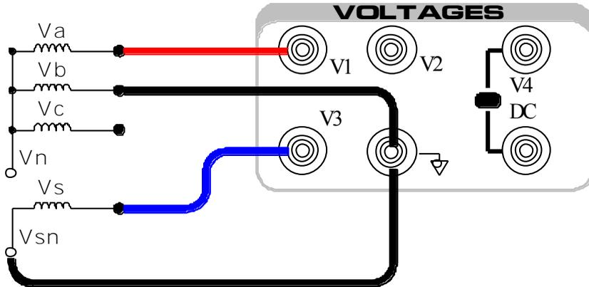
Three Phase Synchronizing Voltage =  $V_{ab}$
