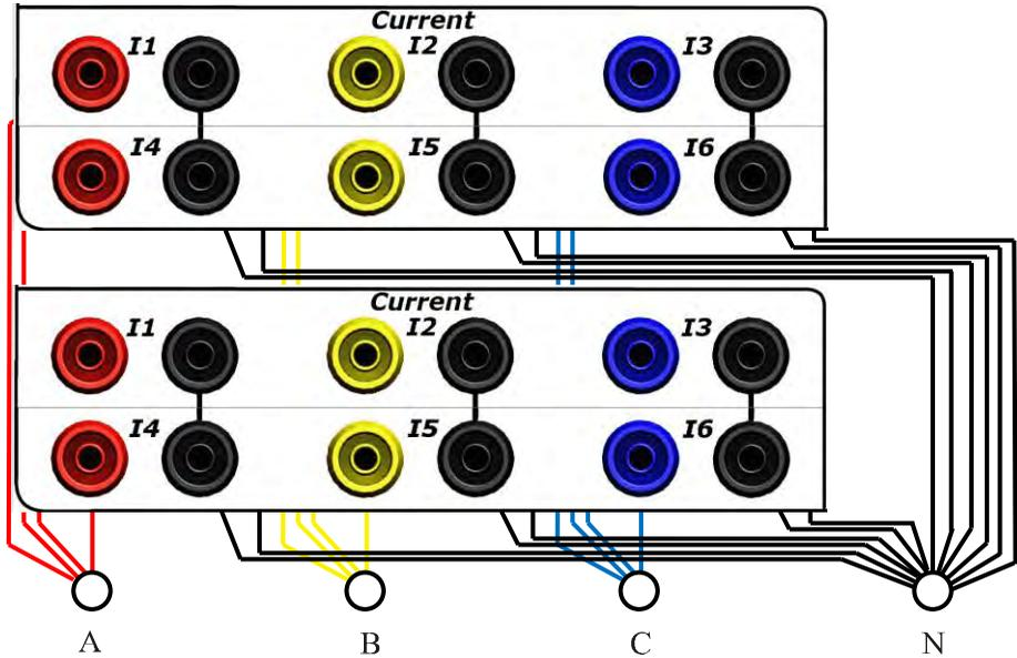
**Figure 8.5 CURRENT CONNECTIONS FOR 3X4 PARALLEL OUTPUTS**
