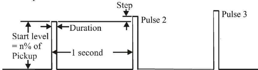
$$\text{Pulse 2} = (\text{Pickup Level} * \text{Start level}) + (\text{Pickup Level} * \text{Step})$$
