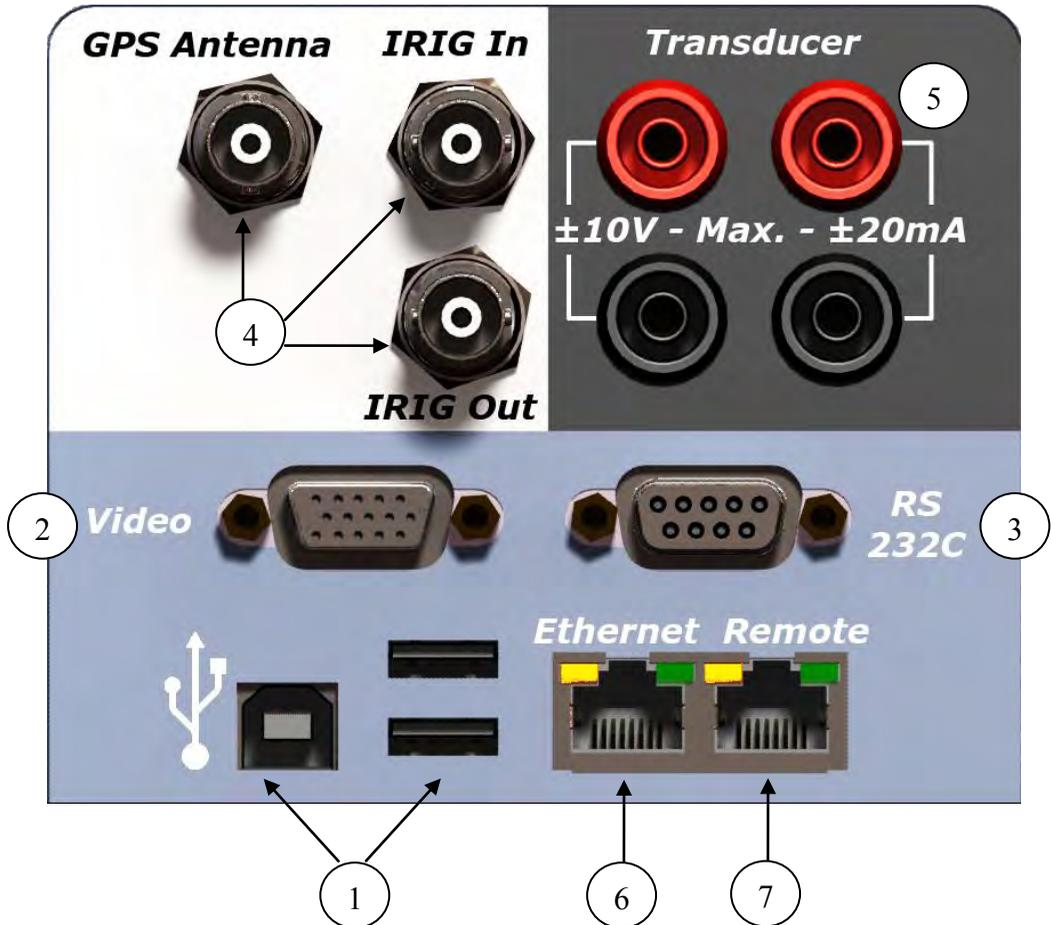
**Figure 3.2 AUXILIARY INPUT-OUTPUTS**
