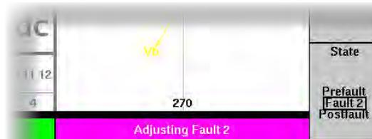
As indicated below, the transition from Prefault to Fault will usually be initiated by a control input to the MTS-5100, and the transition from Fault to another Fault state or Postfault will usually be initiated by the MTS-5100 sensing operation of the equipment under test.
