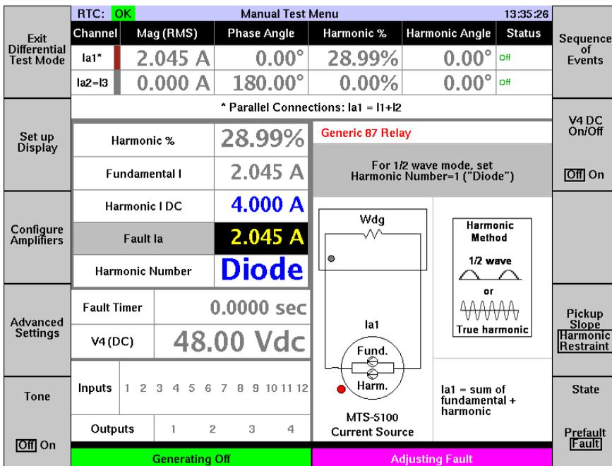
**Figure 3.15 DIFFERENTIAL RELAY HARMONIC RESTRAINT TEST MODE**
