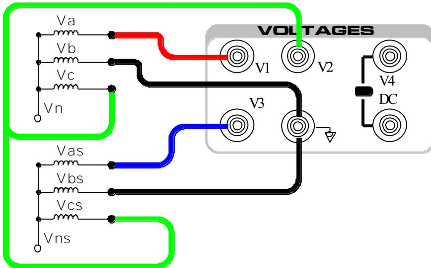
**Synchrocheck Relay: Wiring Type = Delta-Y****Three Phase Synchronizing Voltage =  $V_{an}$**
