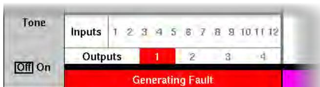
If Timing mode was engaged when the relay under test operates; the status input(s) will be activated, the trip tone will sound briefly, the output channels will switch off, and the timing, voltage, phase, and frequency readings will be frozen. The label below the vector display will state *Captured Fault Values*. The Fault Status box on the display will turn green, display *Generating Off*, and the AC Output Warning LED will turn off. Press RESET to clear the frozen readings.
