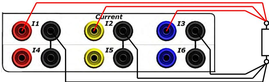
**Figure 3.7 SINGLE PHASE HIGH CURRENT PARALLEL CONNECTIONS**
