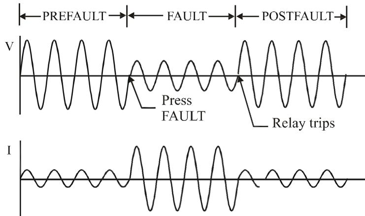
**Figure 4.1 PREFault TO FAULT TO POSTFAULT TRANSITIONS**
