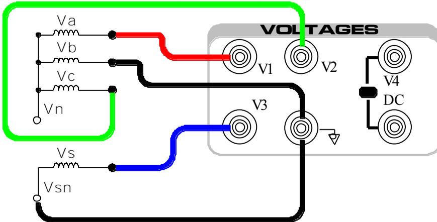
**Synchrocheck Relay: Wiring Type = Delta (cont'd)**
