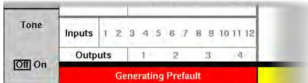
Subsequently pressing the FAULT button will transition the AC/DC output channels to the programmed Fault values. Pressing the RESET button when in Prefault state will turn off the programmed Prefault AC output values.
