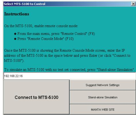
To enable the latter mode on the MTS-5100, first establish a functional Ethernet link and record the IP address of the MTS-5100; see Section 5.3 Ethernet, for details. Enter the IP address on the instruction screen where prompted, and click the Connect to MTS-5100 button. This will bring up the Remote Console display.
