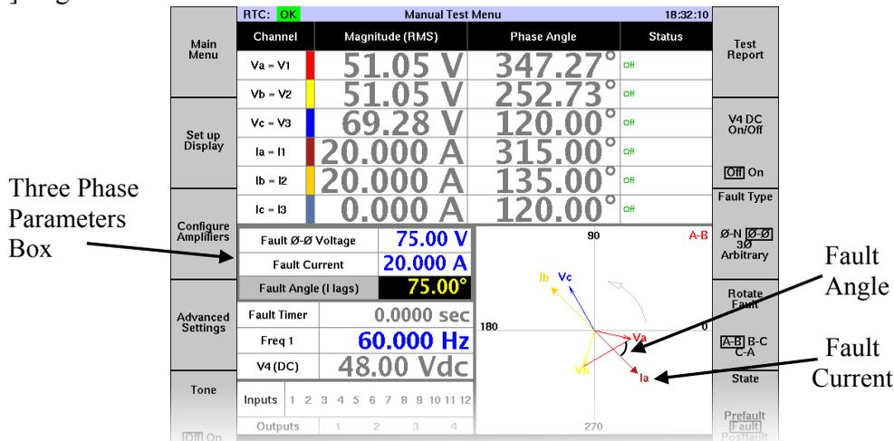
**Figure 4.6 THREE PHASE FAULT CONTROL**
