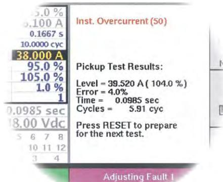
**Figure 3.19 FROZEN OVERCURRENT TEST RESULTS**
