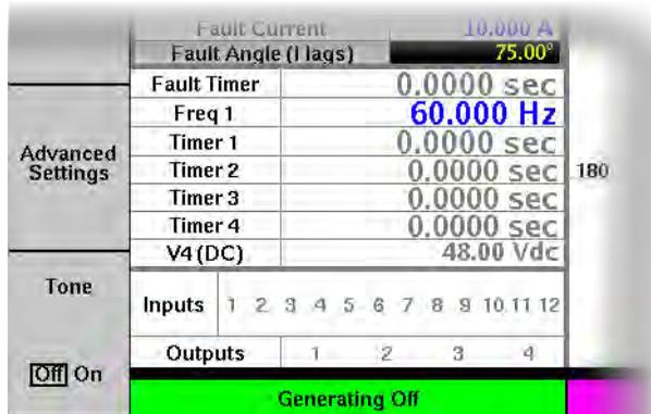
**Figure 4.16 PROGRAMMABLE TIMERS DATA READOUT**
