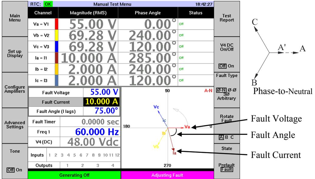
Figure 4.8 PHASE-TO-NEUTRAL FAULT
