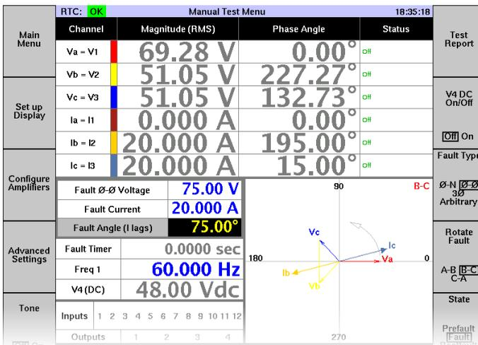
**Figure 4.7 ROTATE FAULT CONTROL**
