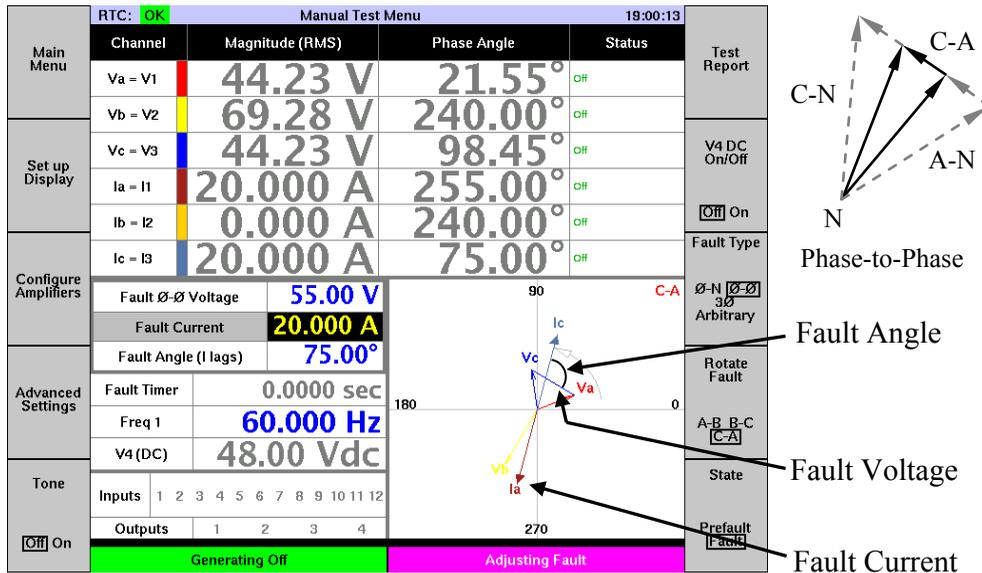
Figure 4.9 PHASE-TO-PHASE FAULT
