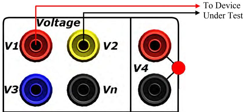
Figure 3.11 HIGH VOLTAGE OUTPUT CONNECTIONS
