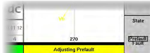
By default, there is 120V phase-to-phase balanced three phase voltage and no current. Enter any desired current, voltage, and phase parameters with the keypad or dial.
