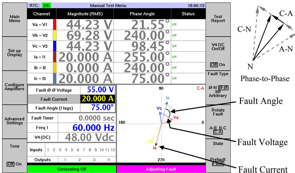
**Figure 4.9 PHASE-TO-PHASE FAULT**
