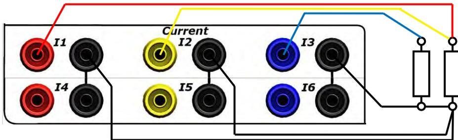
**Figure 3.6 2-CH. MEDIUM CURRENT PARALLEL CONNECTIONS**
