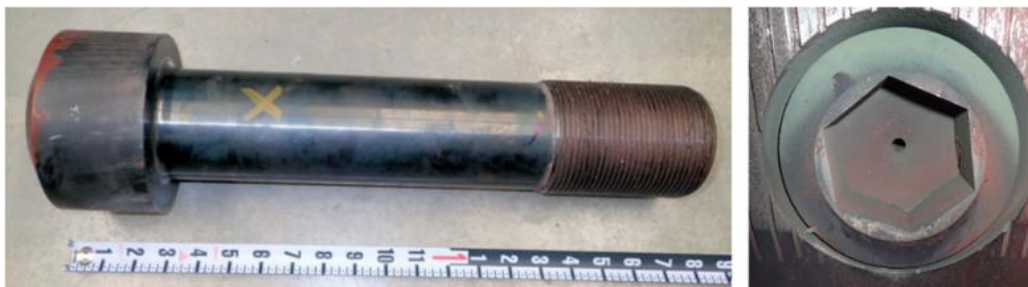
Four Pole – Pole Head Bolt Figure 12
