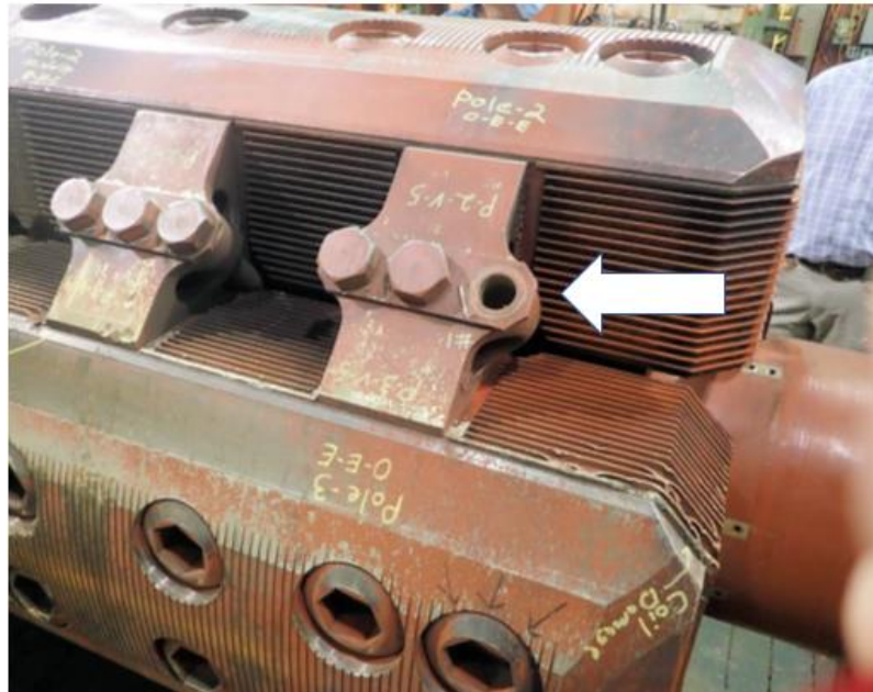
4-Pole Salient Pole Rotor with Removable Pole Top Caps Figure 4
