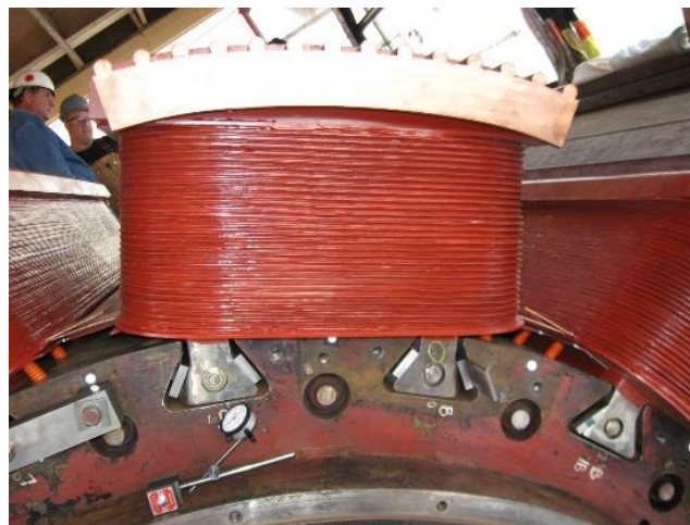
Double Dovetail Root Pole Being Mounted to the Rim of a 10 Pole Rotor Figure 3
