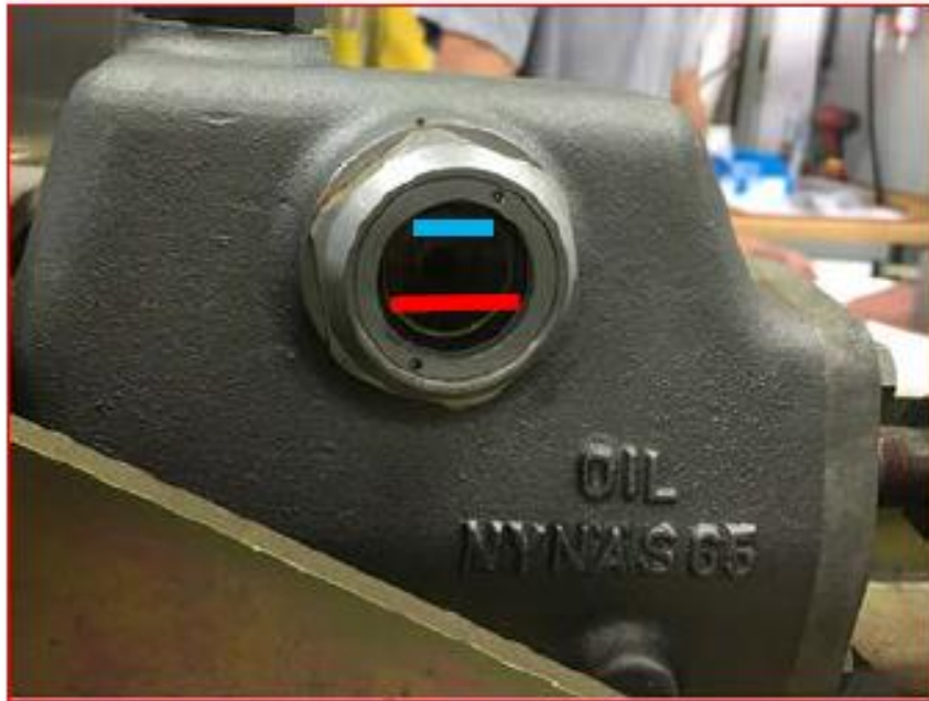
Acceptable Dashpot Oil Level from Service Advisory Figure 3
