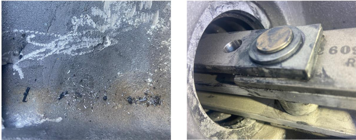
Damage to the Interphase Operating Linkage Seen from Pole 1 Crank Box Figure 7
