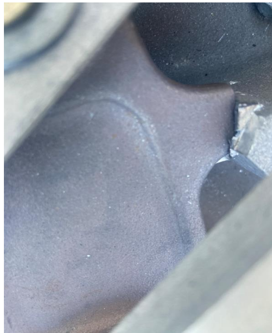
Crank Over travelled into Open Stop Figure 6
