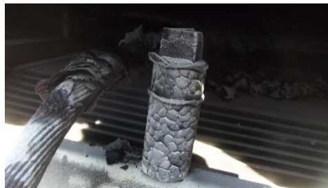
Burned LV Lead, and Core Clamping Structure Figure 2b
