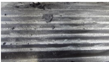
Burned Top Yoke Covered in Fire Soot Figure 2a
