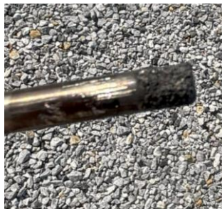
Physical Damage to Bushing Pin Figure 11
