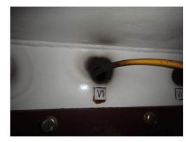
Figure 5 Discharge between unshielded jumper cable and metallic compartment wall.
