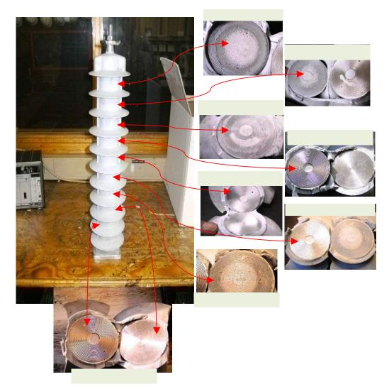
Figure 10. Discharges in a faulty gap arrester.
