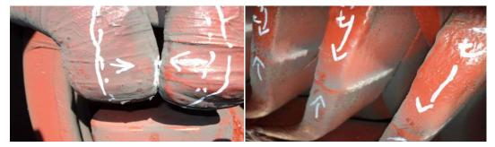
Figure 9 Discharges between phases in the form coil bars and PD from the grading coating.
