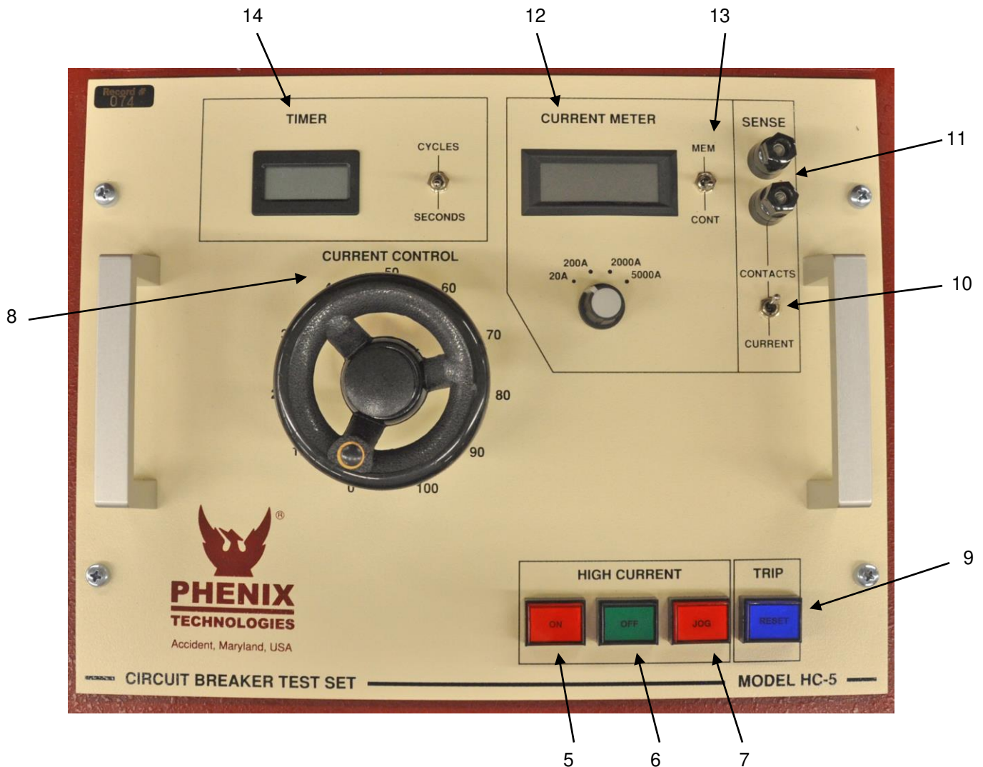
Figure 2. HC-5 Controls and Indicators
