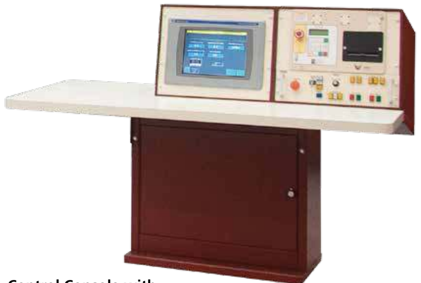
Control Console with rack-mounted Turns Ratio Meter
