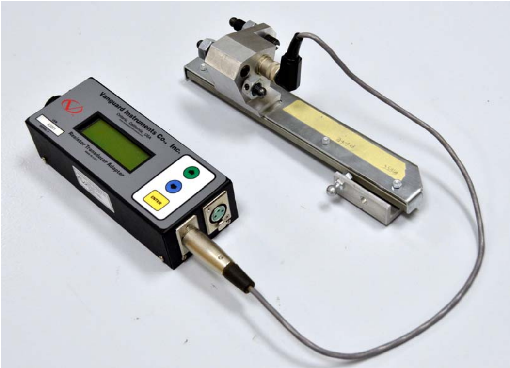
Figure 1. Typical Connection to ABB AHMB Transducer
