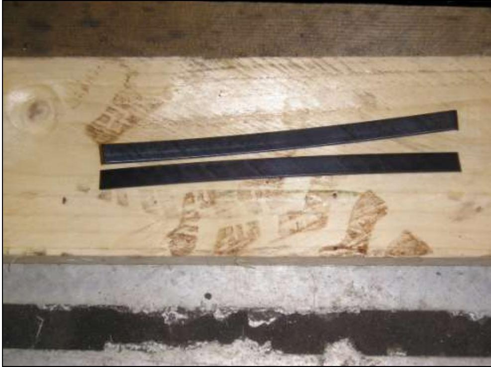
Case Study 3 – Sulphur Corrosion on Conductor Adjacent to Point-of-failure FIGURE 13
