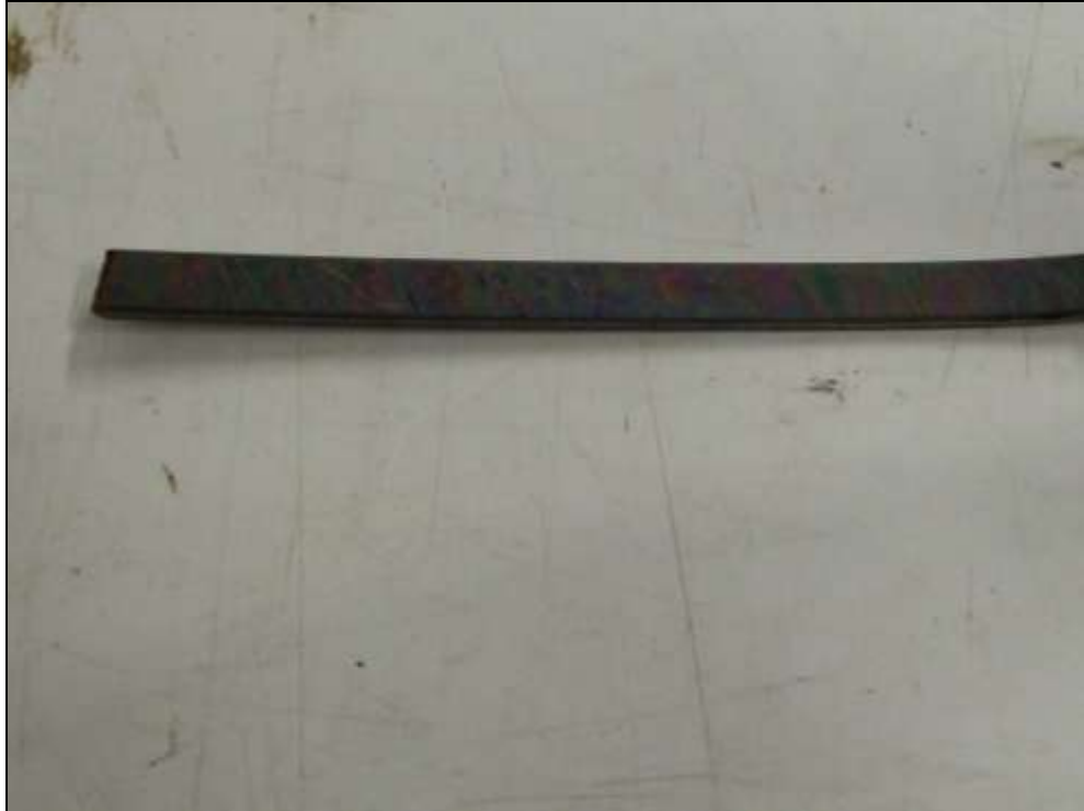
Case Study 1 – Sulphur Corrosion on Conductor from Top Disc of B Phase Series Winding FIGURE 5
