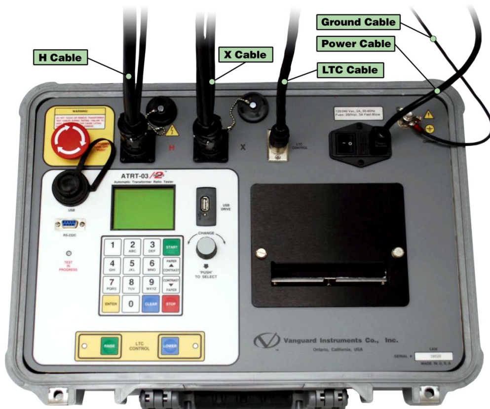
Figure 4. Typical Front Panel Cable Connections
