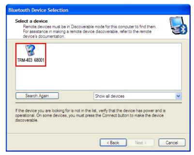
The will will be listed as "UNIT S/N" where UNIT is the name of the unit (TRM-403 in this case) and S/N is the device's serial number. Click on the icon for the unit and then click on the "Next" button.
