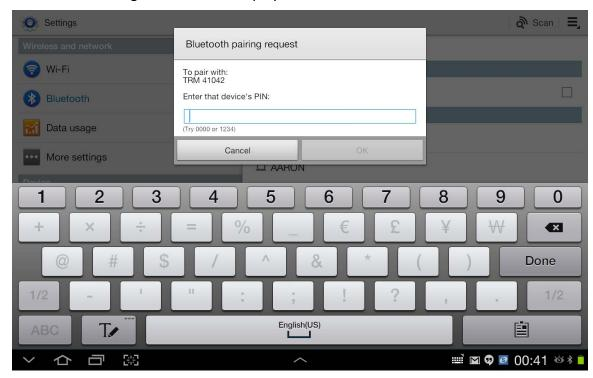
c. The pairing code for Vanguard units is 'default' (without the quotes). By default, only the numeric keys on the on-screen keyboard will be active. To enable alpha-numeric input, slide the dialog box up to reveal the additional options:
