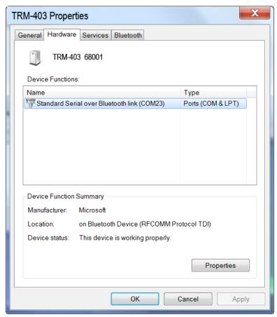
Note the port number listed after the device name (COM23 in the above example). Use this port number in the product's software to connect to the unit.
