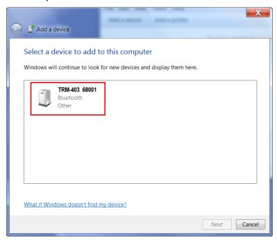
The unit will be listed as "UNIT S/N" where UNIT is the name of the device (TRM-403 in this example) and S/N is the device's serial number. Click on the icon for the unit and then click on the "Next" button.
