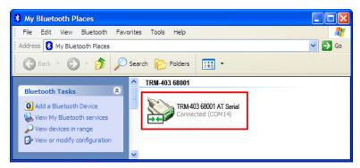
Note the port number listed under the device name. In the above case, the port number is COM14. Use this port number in the product's software to connect to the unit.
