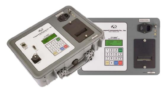
The CT-3500 is Vanguard's second generation, stand-alone, digital, microprocessor-controlled, circuit-breaker timer. It measures the elapsed time from the instant a breaker coil is energized to the instant of opening or closing of a circuit-breaker's dry contacts. In addition to timing a breaker's contact response time, the CT-3500 can also time relays or other switching functions that use an initiating trigger voltage (24-300 Volts DC or AC).
