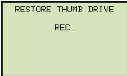
Type the record number that you would like to restore using the alpha-numeric keypad and then press the **[ENTER]** key.
