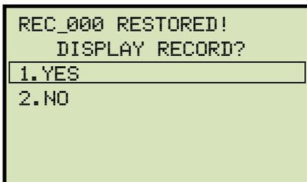
Press the **[1]** key (*YES*) to display the restored test record.
