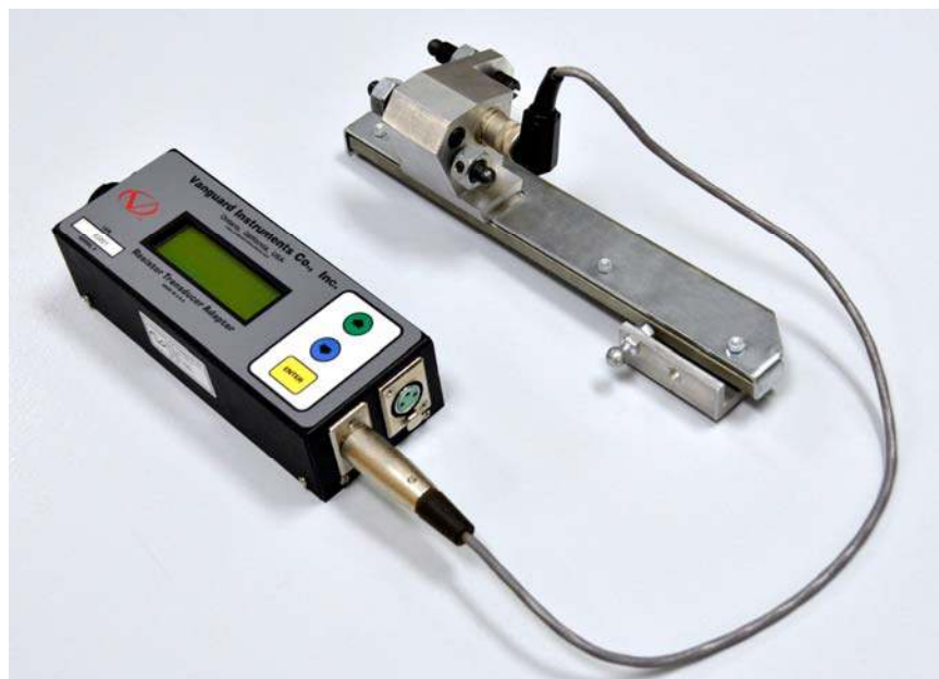
Figure 11. Vanguard Resistor Transducer Adapter Connected to an ABB AHMB Transducer
