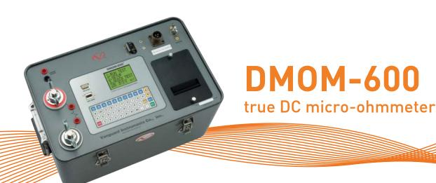
The DMOM-600 is designed to test EHV circuit-breaker contact resistances, bushing contact joints, welding joints, or for any low-resistance measuring application. This high current and very lightweight (33 lbs/ 15 Kg) micro-ohmmeter is designed to meet the IEEE C57.09-1999 (5.15) requirement for testing circuit breaker contact resistance.
