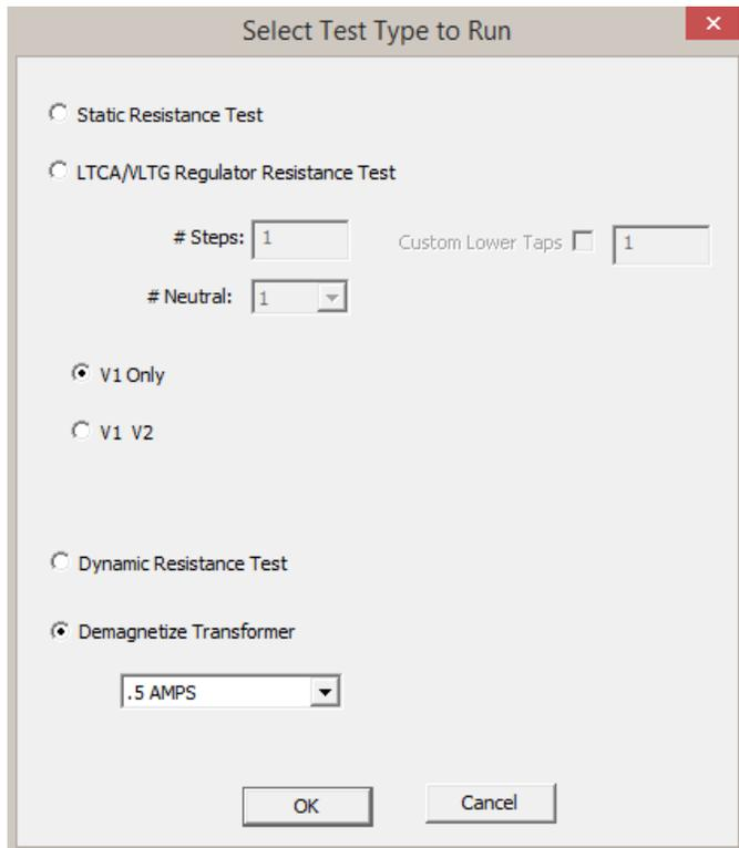
Select the “Demagnetize Transformer” option and select the demagnetization current from the drop down menu below the option. Click on the “OK” button.
