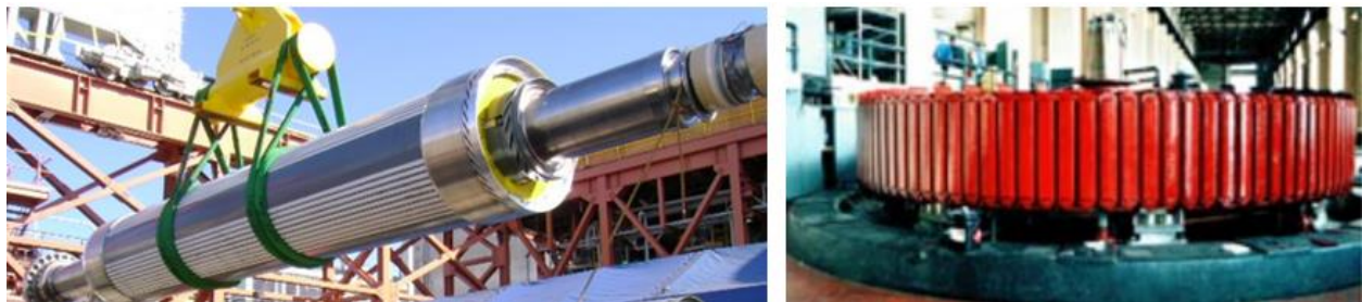
Cylindrical – Turbo Rotor Design (left) Salient Pole – Hydro Rotor Design (right) Figure 13
