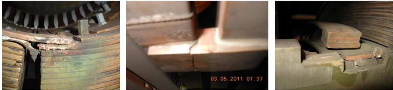
Rotor Pole to Pole Connector Failures Figure 8
