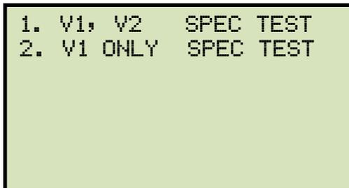
Press the **[1]** key (*V1, V2 SPEC TEST*) to perform a V1 & V2 special resistance test. Continue to step d.
