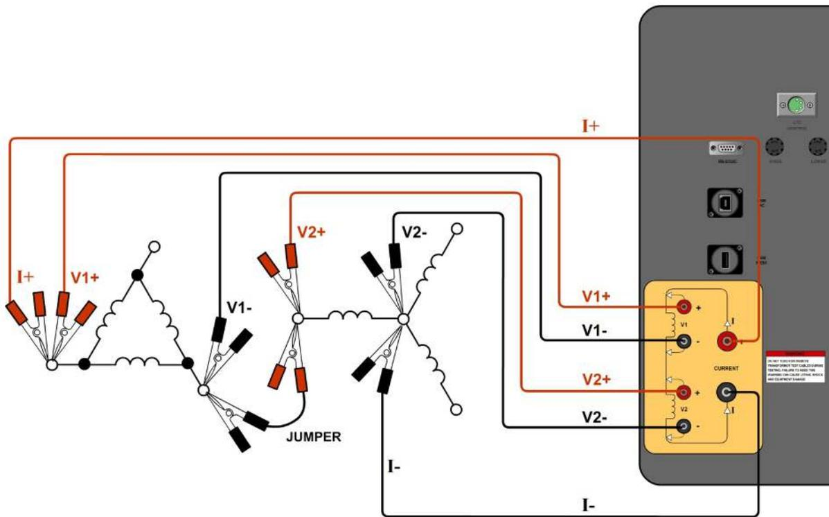
Figure 5. Typical TRM Connections Diagram for 2 Windings
