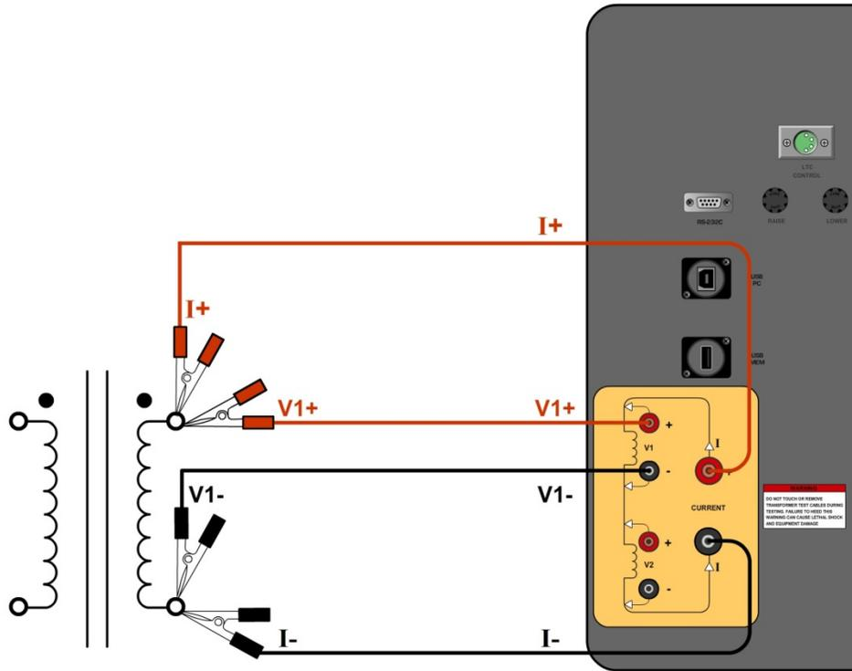
Figure 4. Typical Single Phase TRM Connections
