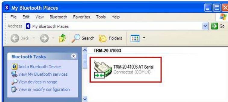
Note the port number listed under the device name. In the above case, the port number is COM14. Use this port number in the LTCA software to connect to the TRM.
