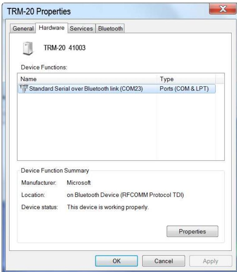
Note the port number listed after the device name (COM23 in the above example). Use this port number in the LTCA software to connect to the TRM.
