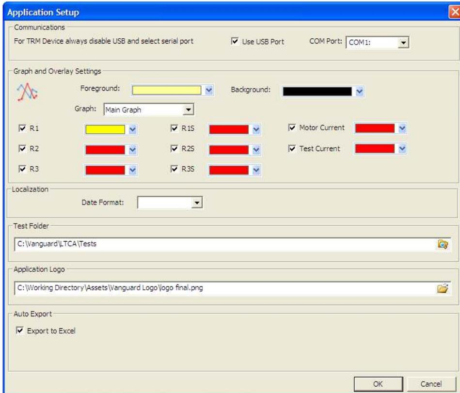
Make sure the “Use USB Port” option is UN-checked. Then, from the “COM Port” drop-down menu, select the COM port that corresponds to the port that the TRM is connected to. Then click the OK button. The LTCA software will now recognize the TRM.
